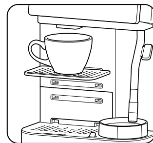
To avoid splatter, use the adjustable cup tray to raise your cup closer to the spouts.
